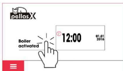
Pic. 2 Boiler start up
